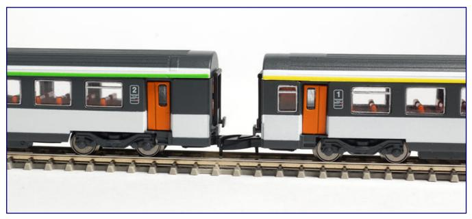
A decisive weak point of the new wagons is the far too great of a distance between the couplers, which is very annoying. Possible solutions could be close couplers or fixed coupling rods, but this needs to be tested at home on the installed radii and counter curves before the wagons are converted for use on the layout.
