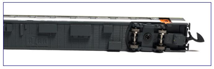
No frills: The wagon floor has no details that would remain hidden from the observer in operation, anyway. The bogies are fastened with screws, which stands in the way of a cable feed-through. The long shaft of the coupling can also be seen here.
