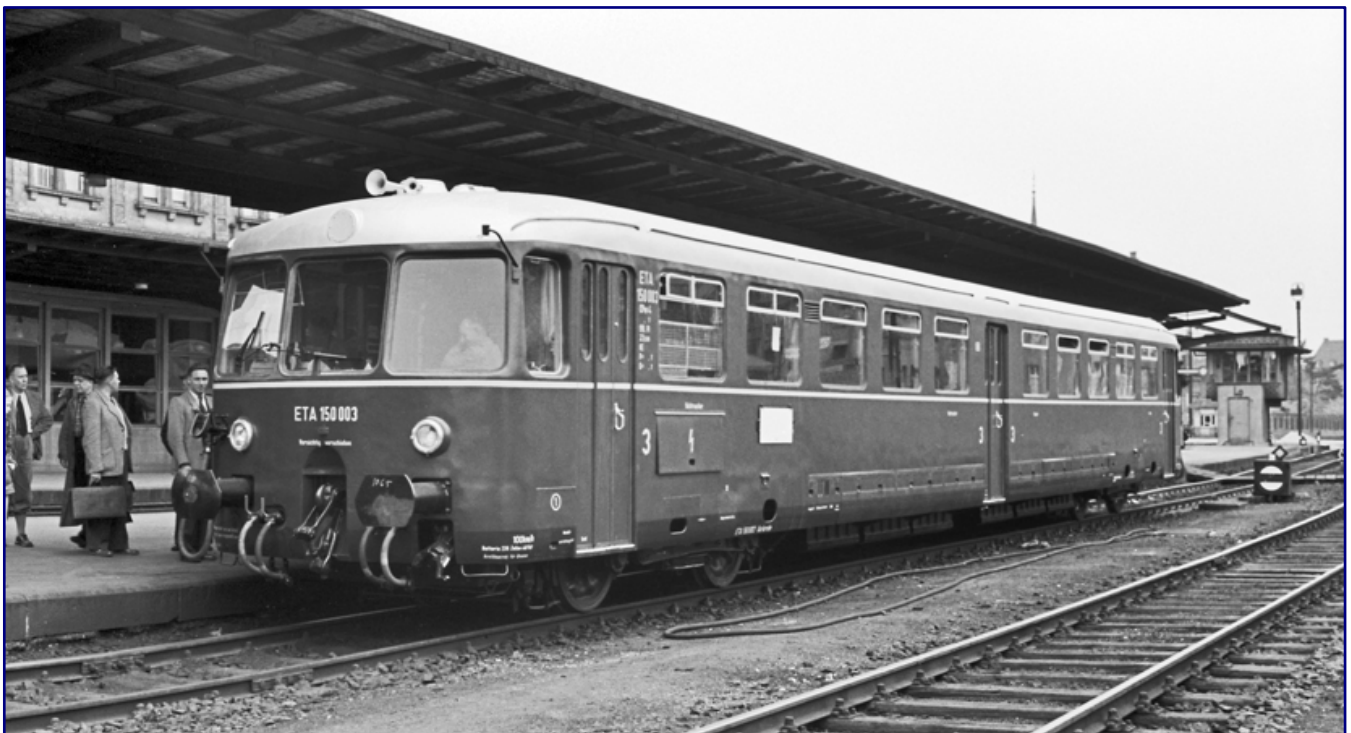
The ETA 150 003 delivered by O&K in Berlin-Spandau in May 1955 was the first production railcar of this series (still without a third headlight). It completed its acceptance test in Limburg/Lahn on 14 May 1955 before entering service at the Basel Bad Bf depot. These vehicles offered passengers a completely new level of comfort. Photo: A. Dormann, coll. W. Löckel (Eisenbahnstiftung)
