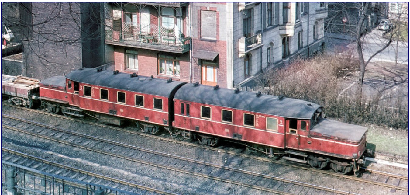
The Wittfeld battery-powered railcars had been in service in Prussia since 1907. ETA 177 101 makes itself useful on its last days in construction train service in February 1963 during electrification work in the Wupper valley. Photo: Carl Bellingrodt, Eisenbahnstiftung
