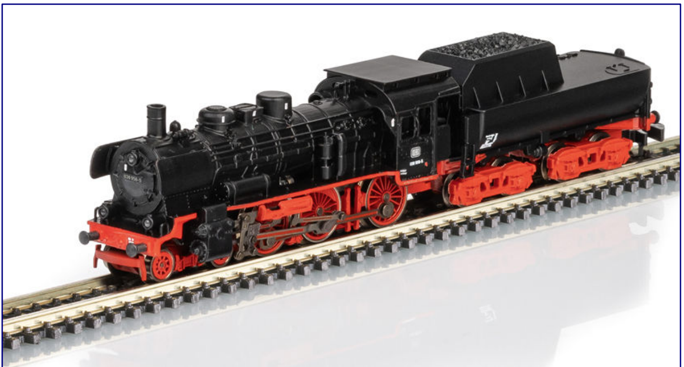
The bronze precision casting gives us Zetties an interesting mould variant of the Prussian P8 as class 038 with tub tender and Indusi equipment (88909). Photo: Märklin
