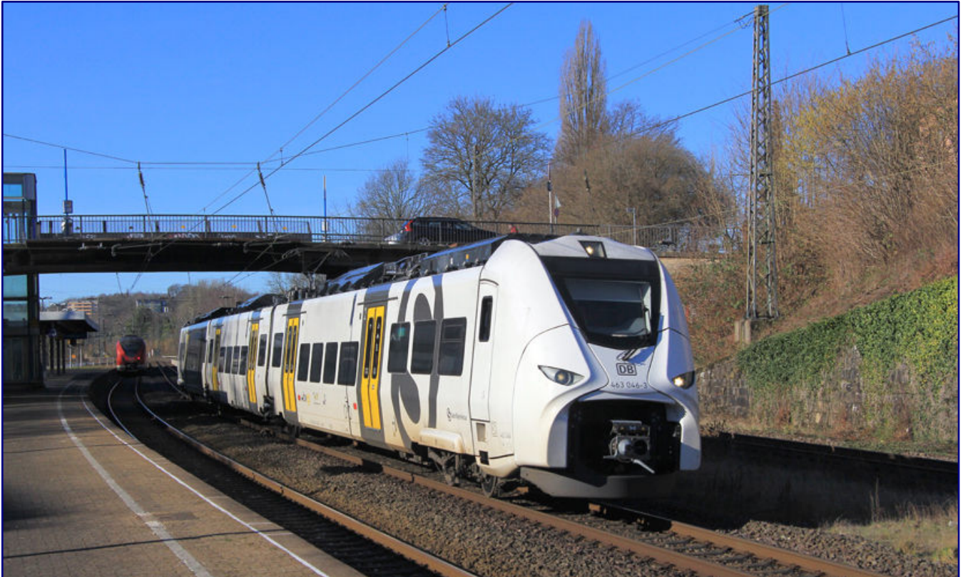
463 046-3 of the S-Bahn Rhein-Neckar, a hybrid train from the Siemens Mireo family, arrived in Wuppertal-Sonnborn on 8 February 2023 as ST 57389 on a test run (Wiesbaden - Minden). At the end of this article, it symbolises the current renaissance of energy storage system powered multiple units. Photo: Wolfgang Bügel, Eisenbahnstiftung
