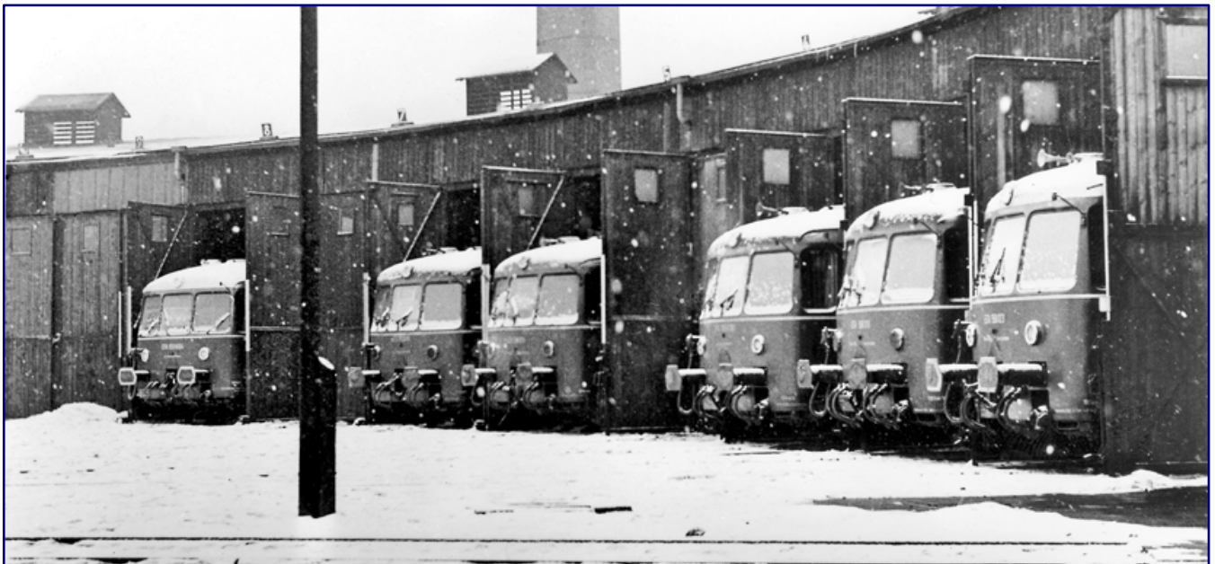
Battery powered railcar parade of the ETA 150 class at the Recklinghausen depot in snowy January 1965. Photo: Willi Marotz, Eisenbahnstiftung
