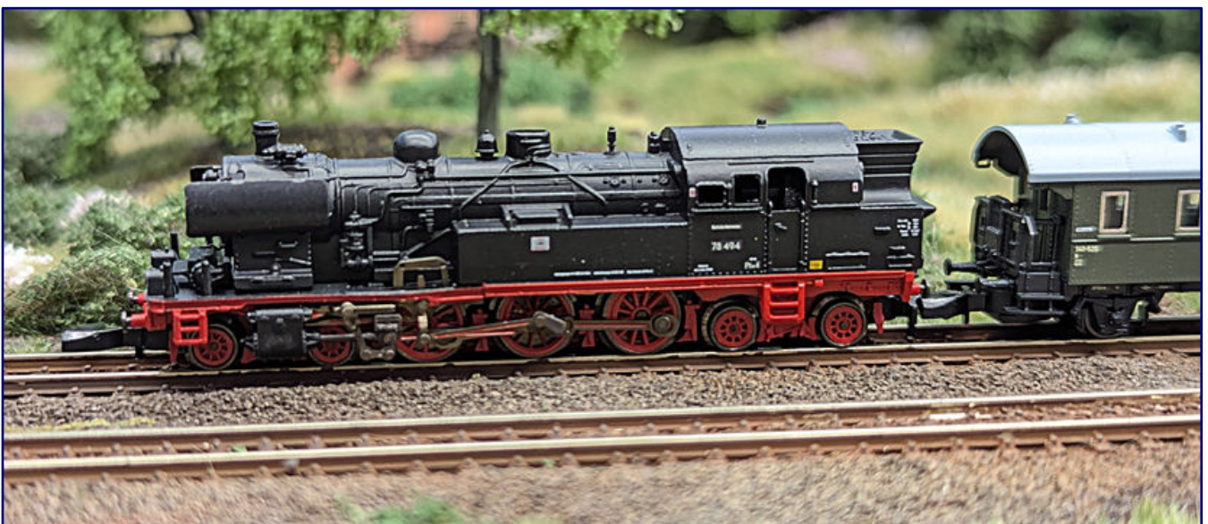
The DR class 78 for operation on Rügen carried Witte wind deflectors (art. no. 88069). Photo; Jörg Erkel | 1zu220-Shop
