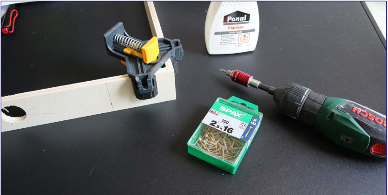
The frames can be fixed and screwed together quite well with a corner clamp.
