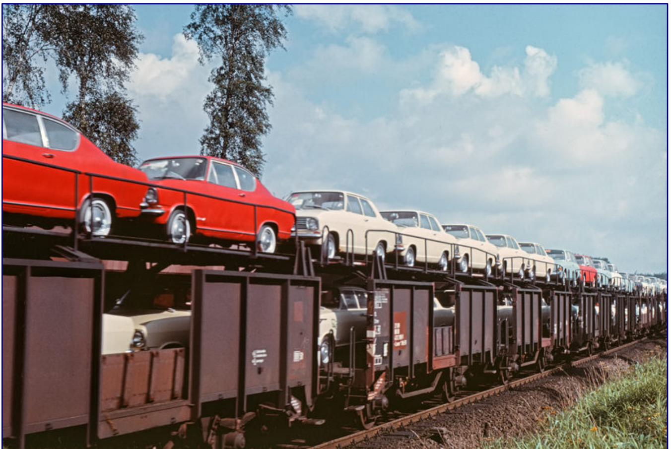
These Opel Kadett Bs, intended for export, were built at the Bochum plant from 1965 to 1973 and are travelling on Offs 59 near Bramstedt in September 1965. At the time the photo was taken, the Off 52, also designed as a provisional solution, was already on its way back. Photo: J.B. Snell, Sammlung Eisenbahnstiftung
