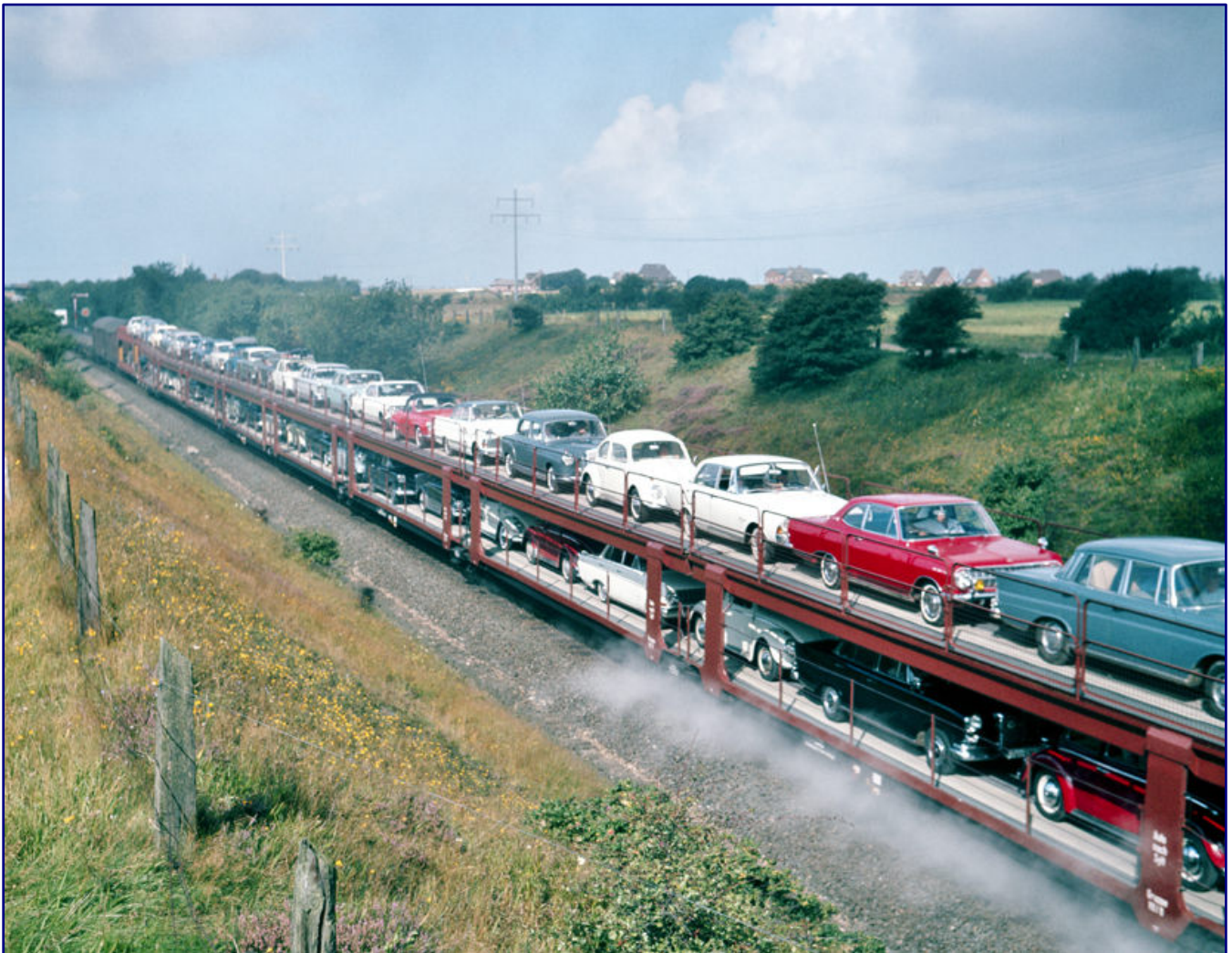
A brief look at the car transport to Westerland in August 1969 near Morsum: A nine-part 'Westerland unit' consists of two end wagons, which correspond to the Laes 547, and seven centre wagons. They replace the previously used two-car Laes 543. Photo: Reinhold Palm, Sammlung Eisenbahnstiftung
