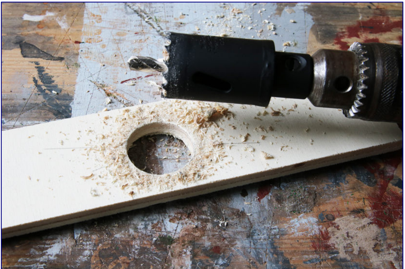
A hole saw, here measuring 26 mm, is used to drill the subsequent wire passages in the frame.
