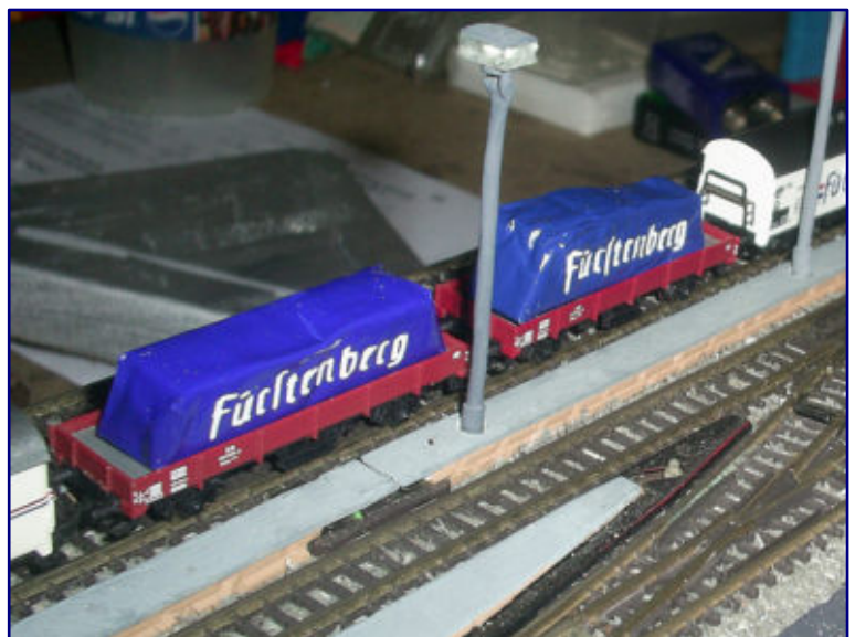
Tarpaulin loads on low-sided wagons created with the help of vinyl film. Photo: Uwe Pfannenschmidt
