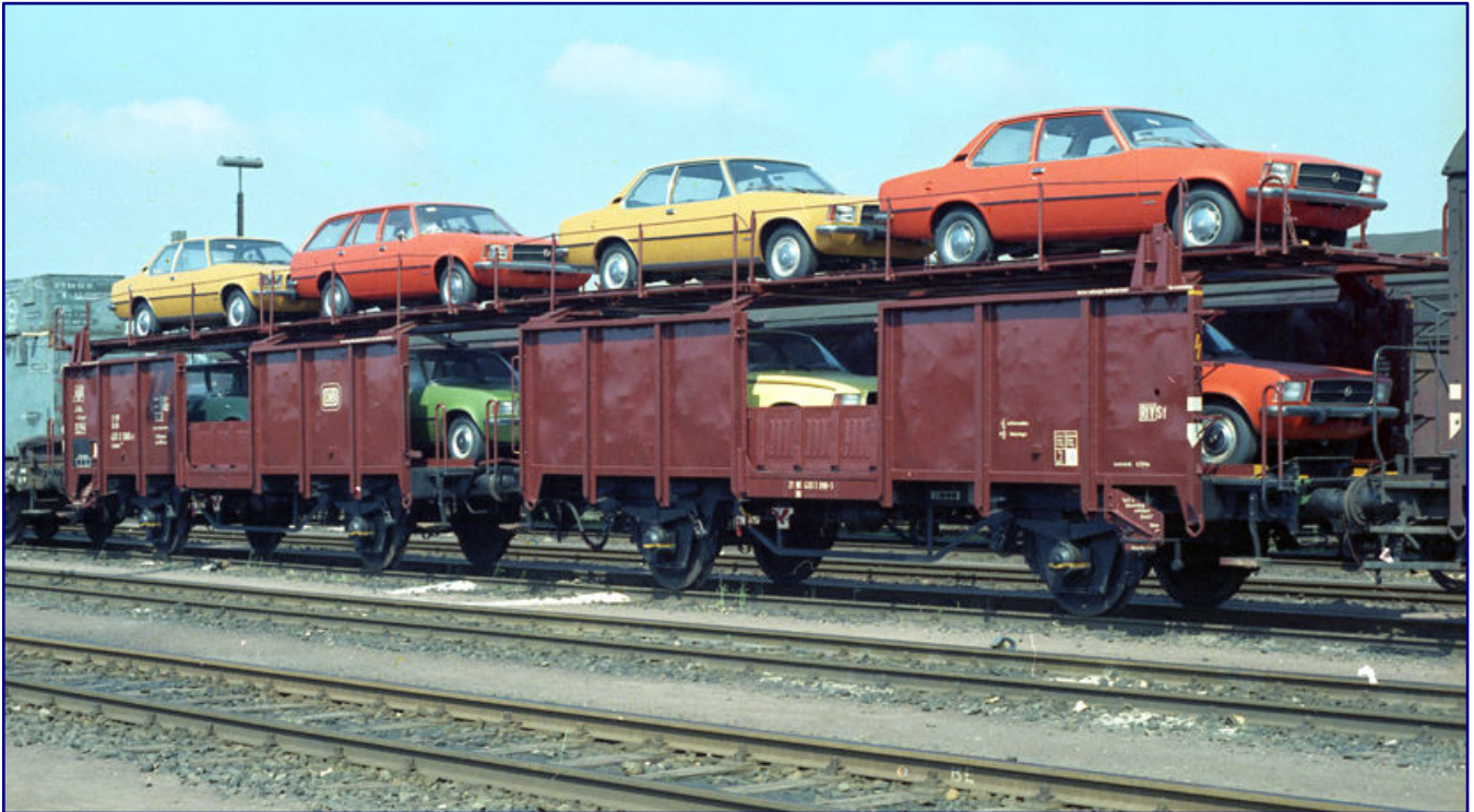
In June 1973, brightly coloured Opel Rekord in Hamburg-Wilhelmsburg on a Laaes 541 (ex Offs 59) waiting to continue their journey. Photo: Benno Wiesmüller, Sammlung Eisenbahnstiftung
