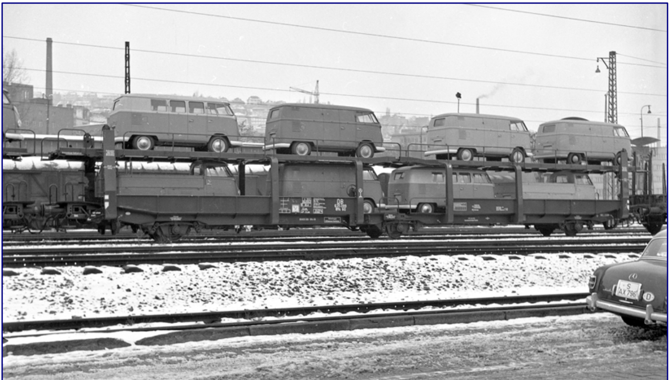
The development of the Off 60 as a third-generation vehicle resulted from the sharp rise in the number of vans and minibuses being transported at the end of the 1950s. Photo: Fritz Willke | © Stefan Carstens
