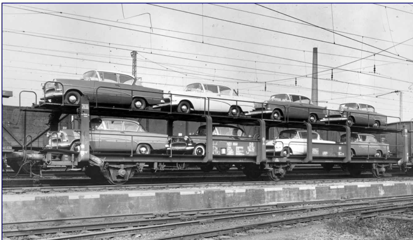
The top photo from Untertürkheim station shows an Offs 55 (Laes 542) in its modified design with half-height sheet metal side walls; for comparison, the photo below shows the original design again. Photo: Fritz Wilke | © Stefan Carstens (top photo) & Carl Bellingrodt | Slg. Stefan Carstens (bottom photo)
