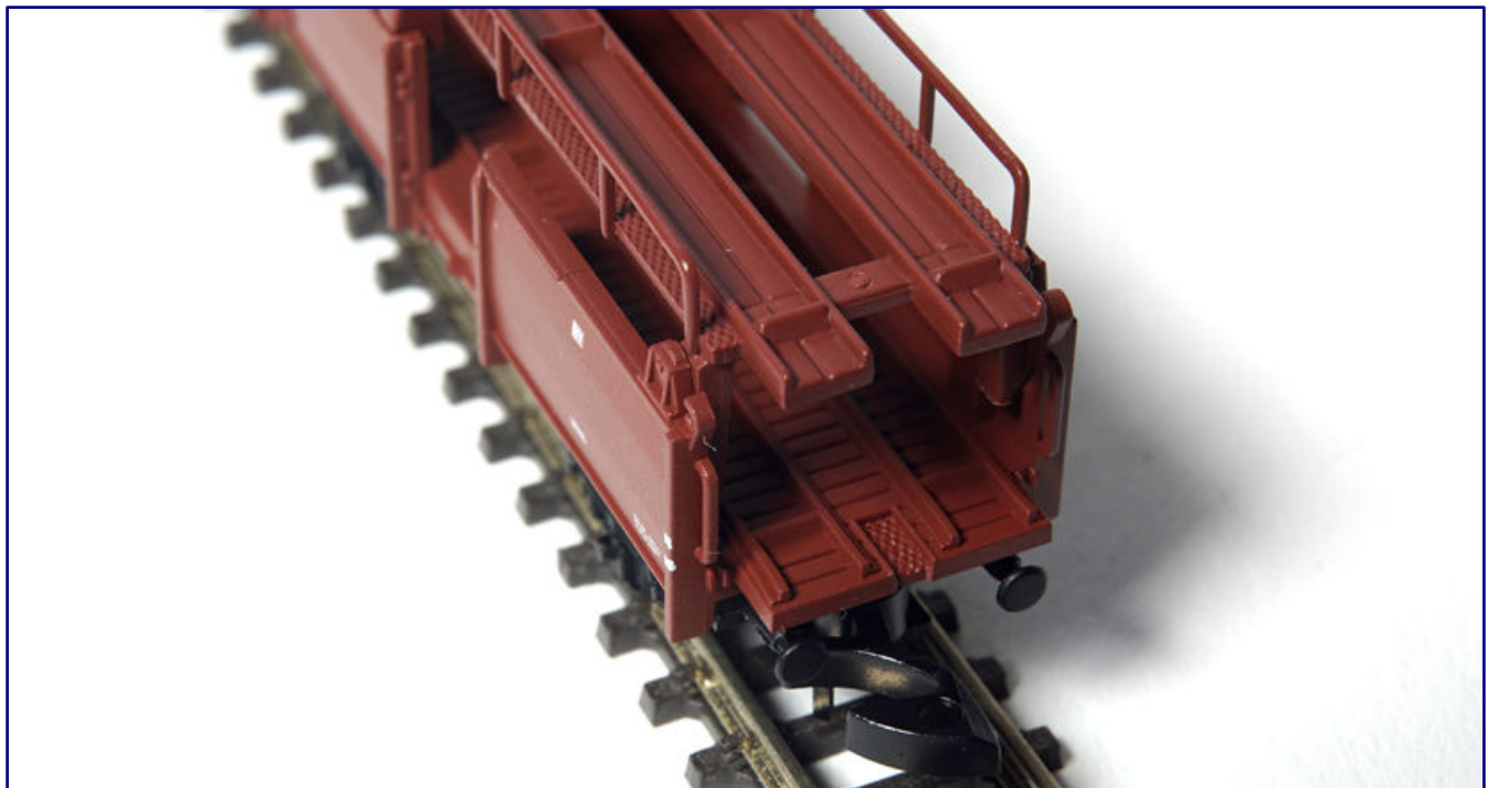
The top view shows the wooden covering of the wagon floor and the recesses of the loading platform, each with locking rails and wheel chocks.
