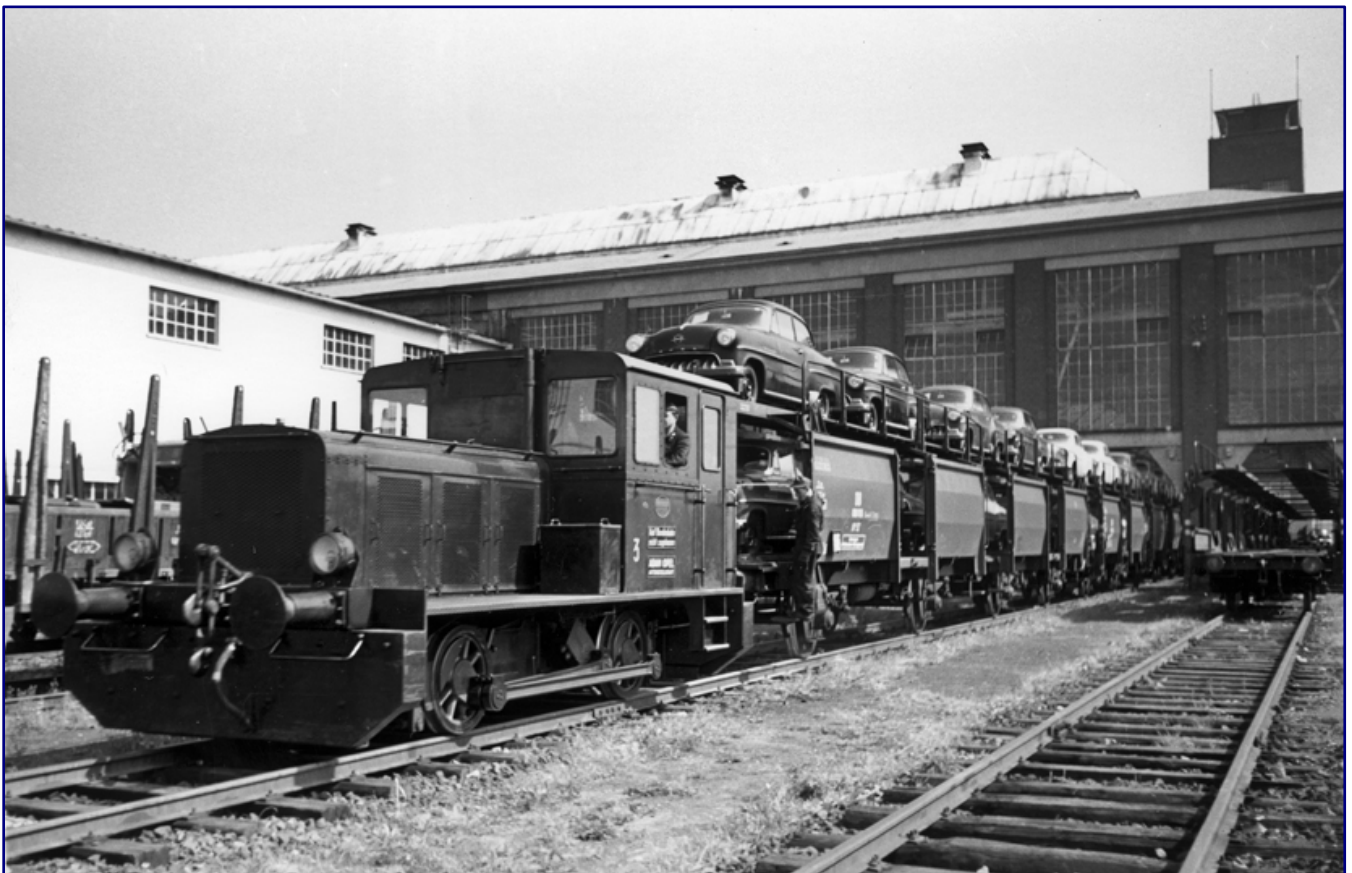
Factory locomotive 3 of Adam Opel AG pulls a line of Off-52 wagons loaded with Opel Olympia Rekord from the Rüsselsheim factory halls in 1954. Photo: Sammlung Stefan Carstens
