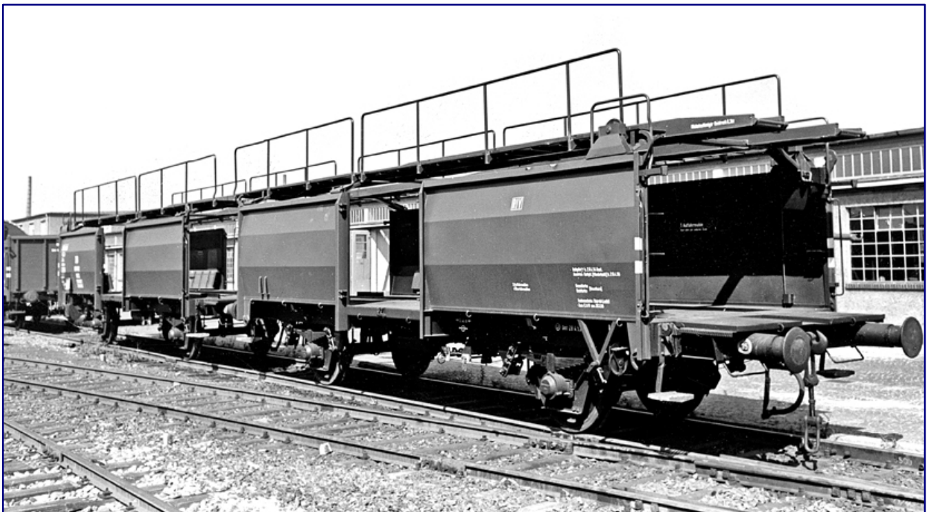
This photo of an Off 52 double unit supposedly dates back to 1960. The railings on the loading platform have long since been retrofitted, but strangely enough there is no sign of the locking rails for fixing the shell wheel chocks in the lower deck. Photo: Bustorff, Sammlung Eisenbahnstiftung.
