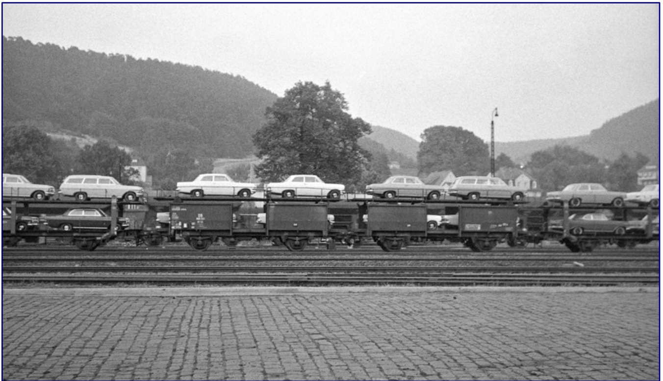
The Off 52 double units were unmistakably derived from the Omm 52 open goods wagon and could therefore be recognised as a provisional solution, which, however, performed perfectly well and was accepted by the car manufacturers. Photo: Dr. Rudo von Cosel | © Stefan Carstens
