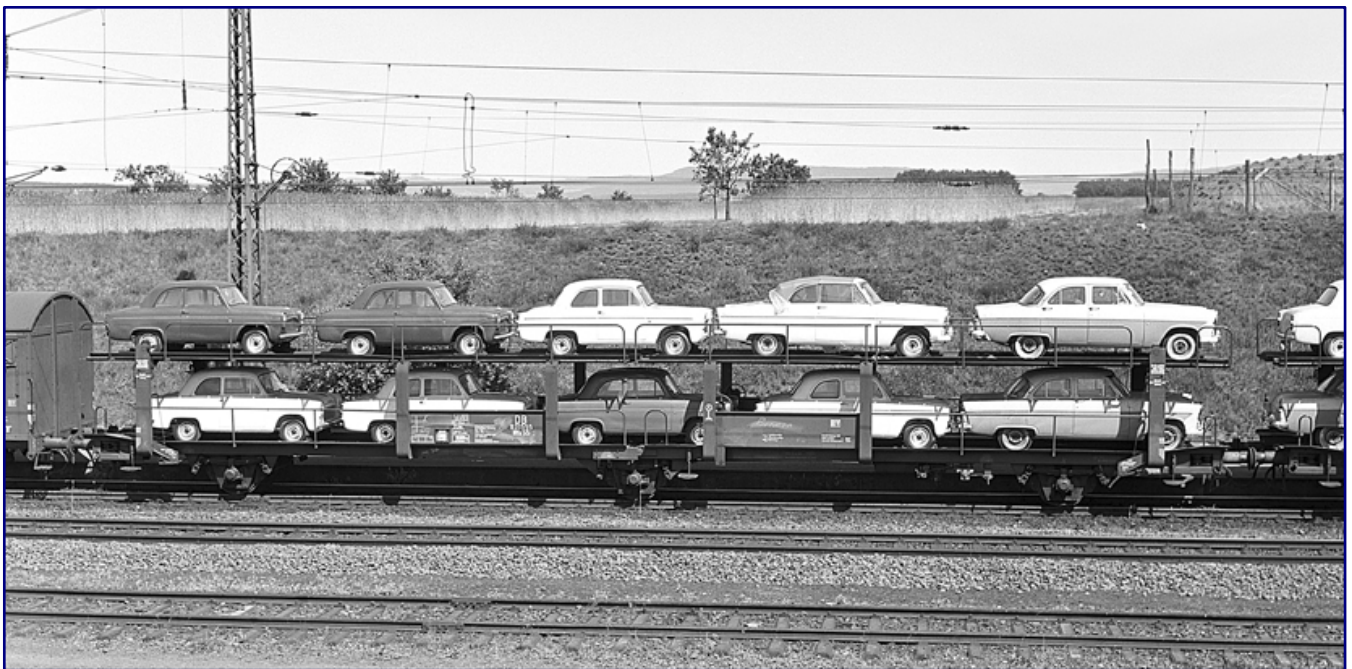
This photo taken near Nuremberg on 5 June 1959 shows a loaded Offs 55 in its original design with sheet metal panels and railings on the lower deck. Photo: Joachim Claus, Sammlung Eisenbahnstiftung
