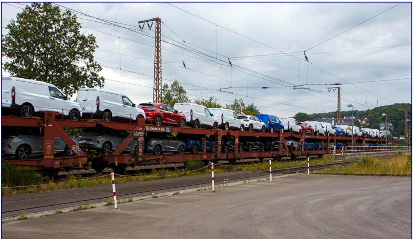
Here, a Laeeks 553 of DB Cargo Logistics GmbH (ex DB Schenker ATG) is seen on 1 August 2024 in a train formation passing through Wilnsdorf-Rudersdorf (Siegen district). The wagon with the road number 25 80 4367 693-5 D-ATG was built by Waggon-Union Berlin in 1988 and was transferred to ATG by the Bundesbahn. Photo: Armin Schwarz
