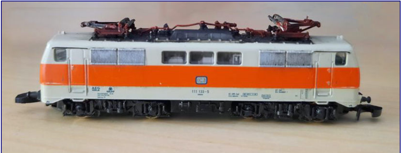
Our reader has reworked this class 111 locomotive so that the single-arm pantograph, which is not extended, lies flat on the roof and does not look too oversized. Photo: Michael Fuhry
