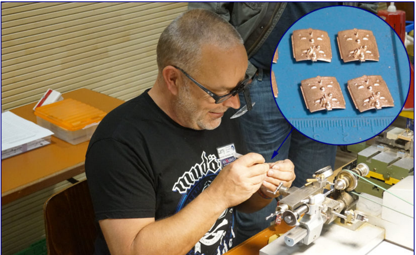
Ronald “Larry” Schulz demonstrated precision mechanical work. The customers were able to see the necessary reworking of cast replacement roofs for Märklin’s V 60 (see picture), where the cast burrs were removed.
