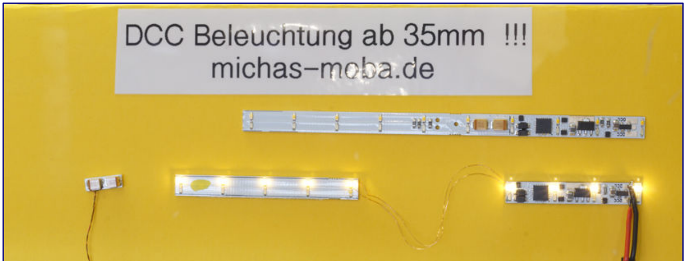
At the Dietmar Allekotte stand, Michael Boost presented his new DCC interior lighting for passenger coaches in the display case. As it can be individually shortened down to a length of just 35 mm, it can be used in a wide variety of models.
