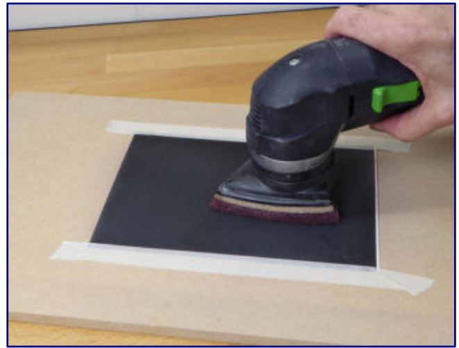
Vinyl film is tarnished by hand using a sanding fleece (photo left) or with the help of a delta sander (photo right).
